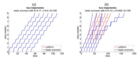
Fig. 6. Effect of small positive (a) and negative (b) deviations from  $b_{crit}$ ; no exogenous delay
