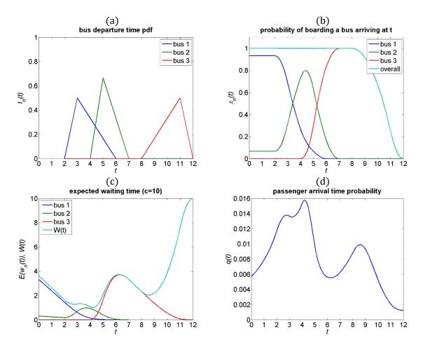
Fig. 2. Illustration of the reliability-based passenger arrival model
