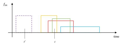
Fig. 1. Example of bus arrival probability distributions functions at a stop
